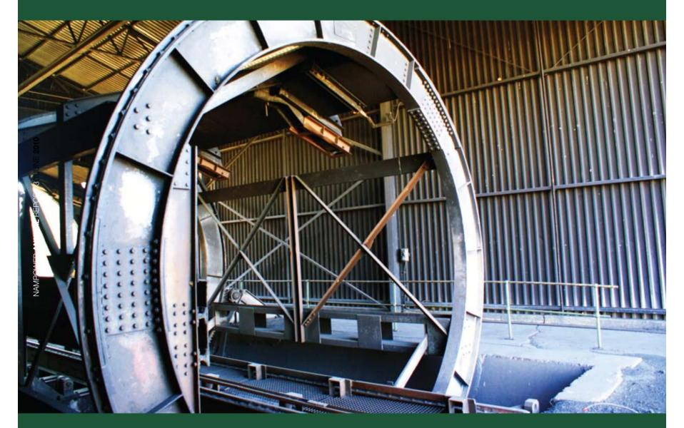
Rotary wagon coal tippler at Van Eck Power Station
