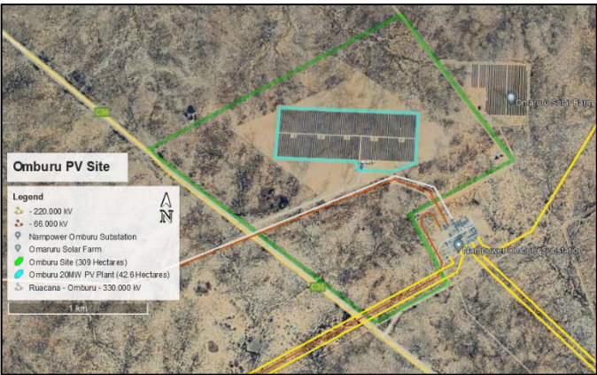
Figure 2: 80 MW Omburu PV II Project site location
