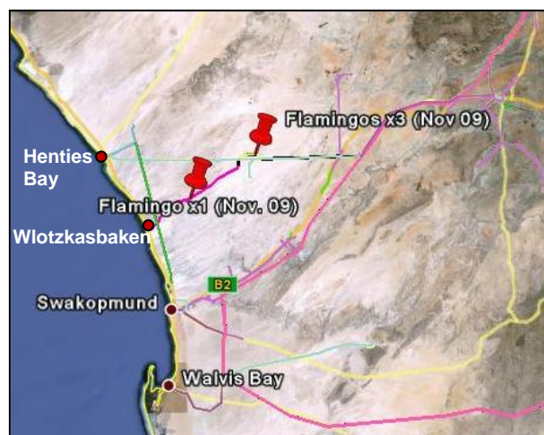
Google image showing sites of flamingo collisions (red markers) on the new 132 kV Trekkopje-Wlotzka line north-east of Swakopmund (left), and 66 kV Trekkopje Bypass (right) (based on a Google map generated by Alice Jarvis [EIS]).
